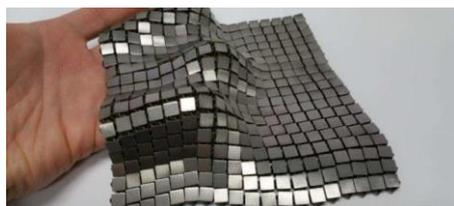
Engineers at NASA's Jet Propulsion Laboratory (JPL) created a 3D printed metallic fabric that can be used in space. The silver, strong fabric was 3D printed in one piece, and has four functional properties: reflectivity, foldability, passive heat management and tensile strength. <https://materia.nl/> Texto y fotos: materia. 5 Mayo 2017.
