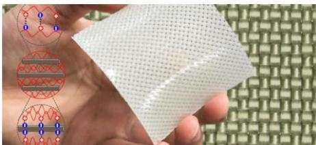
A hydrogel is a superabsorbent gel made of natural or synthetic polymers. They can absorb up to 99.5 per cent water in volume. Because they can be made from natural polymers, the substance has potential as a structural biomaterial. Researchers at Hokkaido University (JP) created fibre-reinforced soft composites, or a tough hydrogel combined with woven fibre fabric. The new material is highly flexible, tougher than metals,
