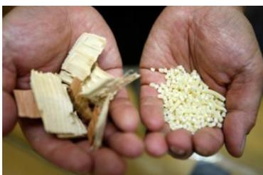
With the rapid development of electric cars, finding a lightweight material to replace steel is more important than ever in the automotive industry. Japanese researchers and auto suppliers are working with what would appear to be an unlikely substitute: wood, or more specifically, cellulose nanofibres. According to the researchers, a material made from wood pulp is 5 times as light and can be 5 times as strong as steel. <https://materia.nl/> Texto y fotos: materia. Octubre 2017.
