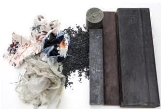
Wootex is a new material made of recycled textile and plastic waste, produced in a unique, patented process. It offers 'woodlike' qualities and is an environmentally friendly, easy to process and low-cost material. Ideal for manufacturing noise barriers, beams, flowerboxes, garden patios and just about anything builders, designers and manufacturers can come up with. <http://blog.is-arquitectura.es> 17. Texto y fotos Blog de arquitectura.es. 29 Junio, 2017
